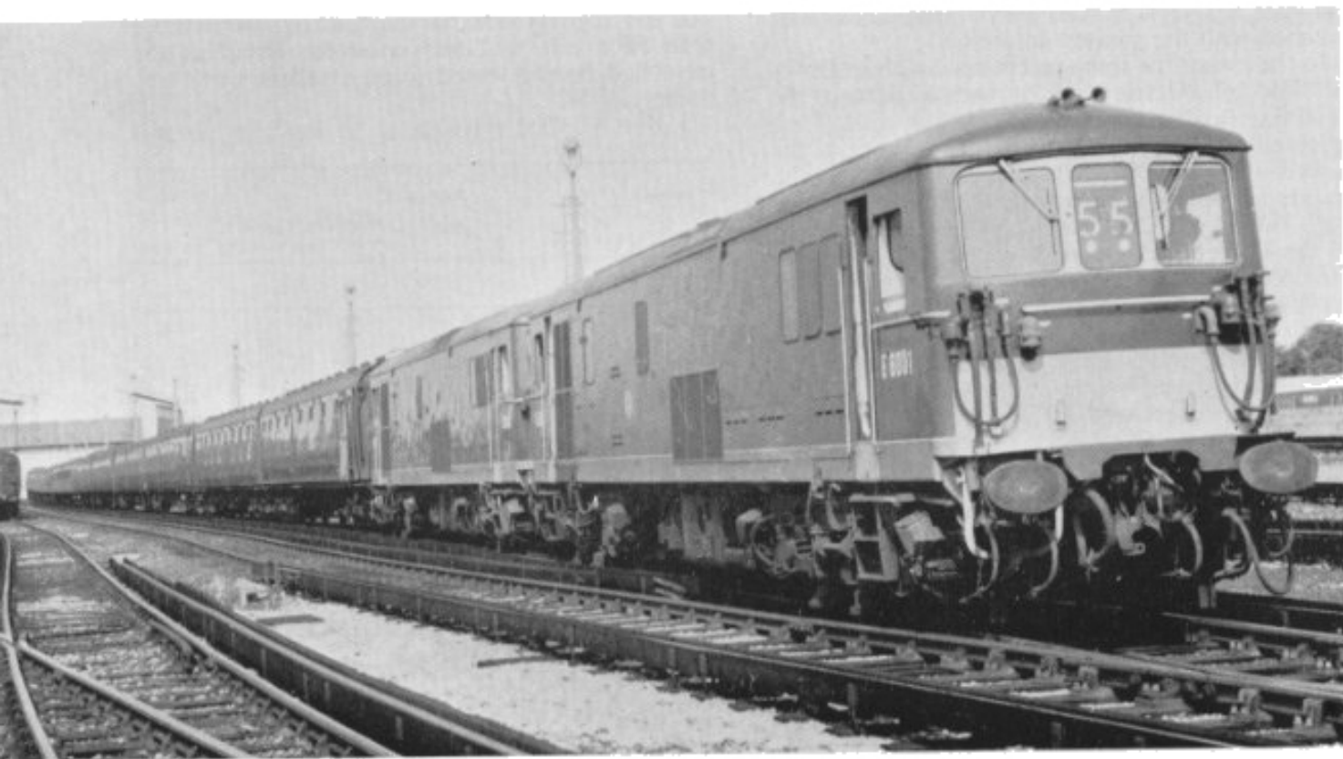
Train used for second series of propulsion tests by the Southern Region of British Railways, worked by electro-diesel locomotives Nos. E6001 and E6006
