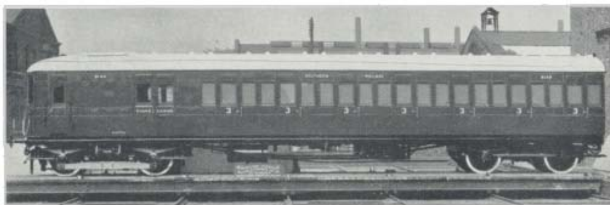
Steel-panelled motor coach, built for the Western Section in 1925
