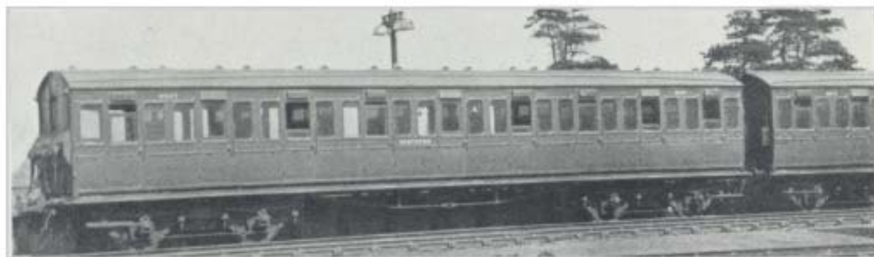
Nine-compartment trailer vehicle, converted from L.B.S.C.R. steam stock
