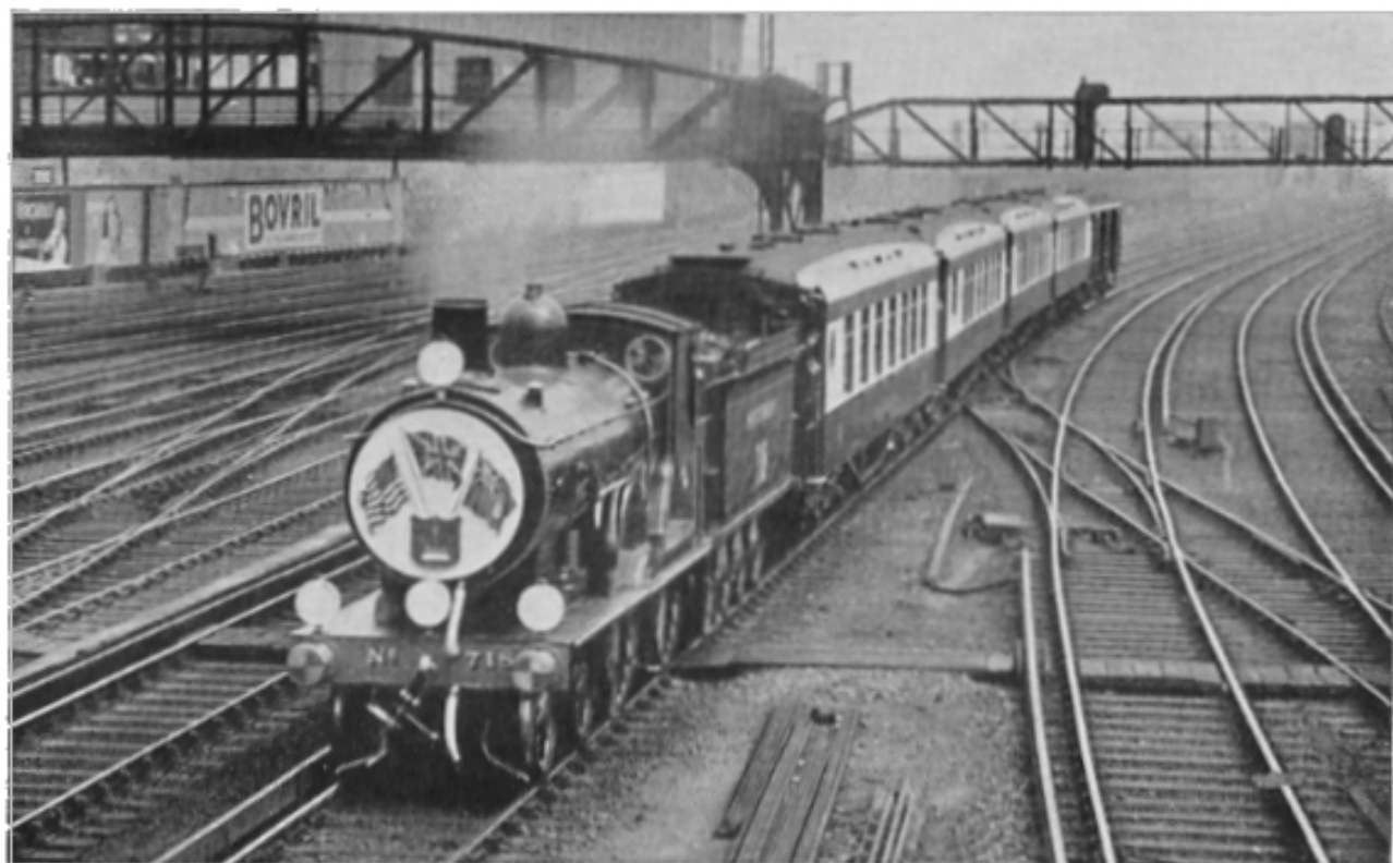
Royal Train approaching Clapham Junction, Southern Railway, on May 6, 1939 Drummond "T9" class 4-4-0 locomotive No. 718
