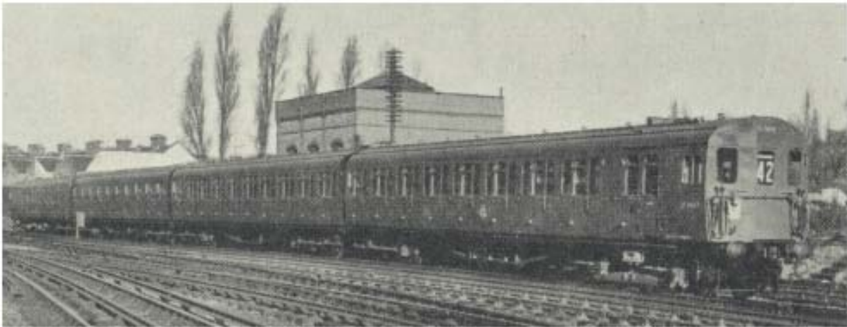
Rebuilt Southern Region multiple-unit suburban train fitted with new standard electrical equipment
