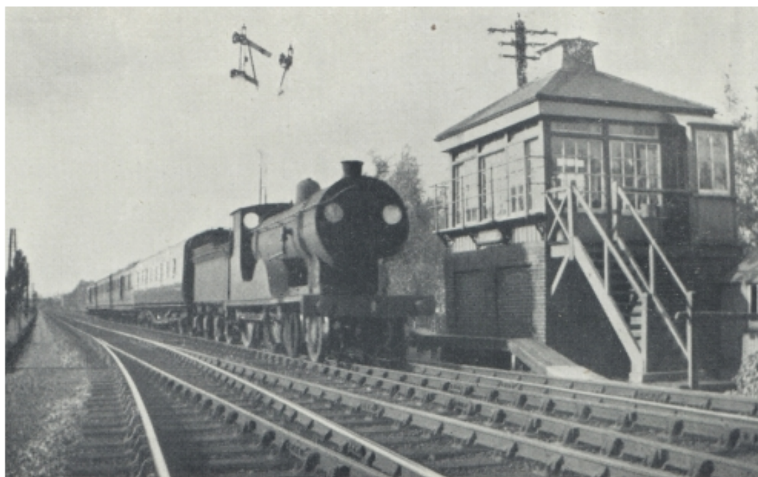
Photo [H. M. Madgwick] Bournemouth to Portsmouth train passing Cosham Junction, hauled by Drummond "L12" class 4-4-0 locomotive No. 30433
