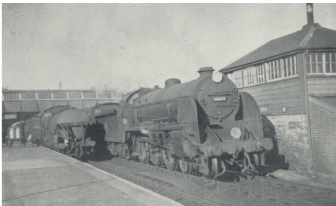
Photo [R. S. Morton] Exeter train at Axminster Station, headed by "S15" class 4-6-0 locomotive No. 30824
