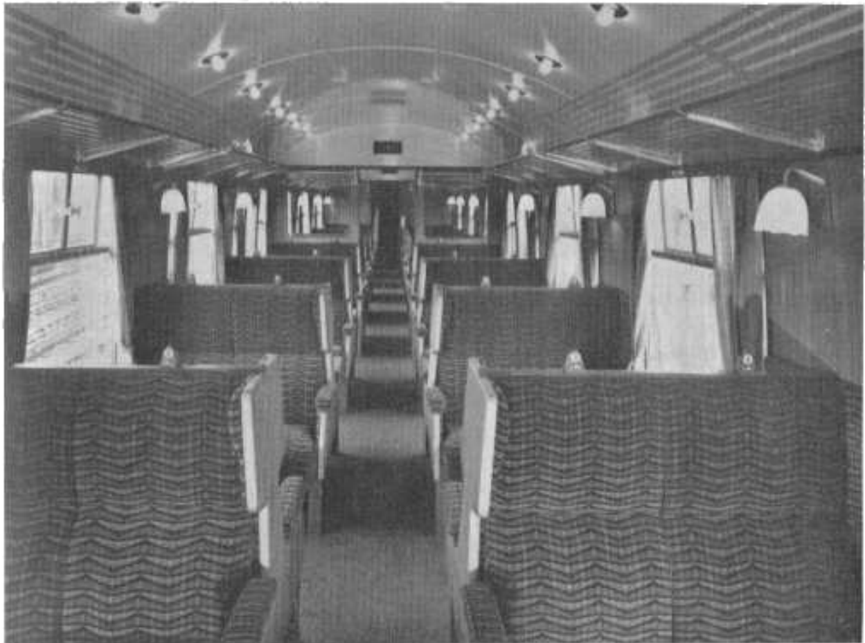
Saloon of the second class motor coaches at each end of the sets which contain a guard's and luggage compartment. The other two coaches comprise a corridor second (or kitchen buffet car) and a corridor composite
