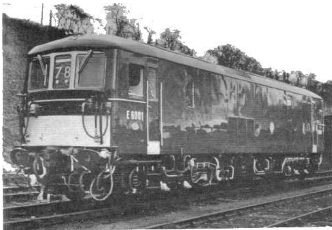
No. E6001, the first of the six dual-power experimental locomotives being built at Eastleigh for the Southern Region
