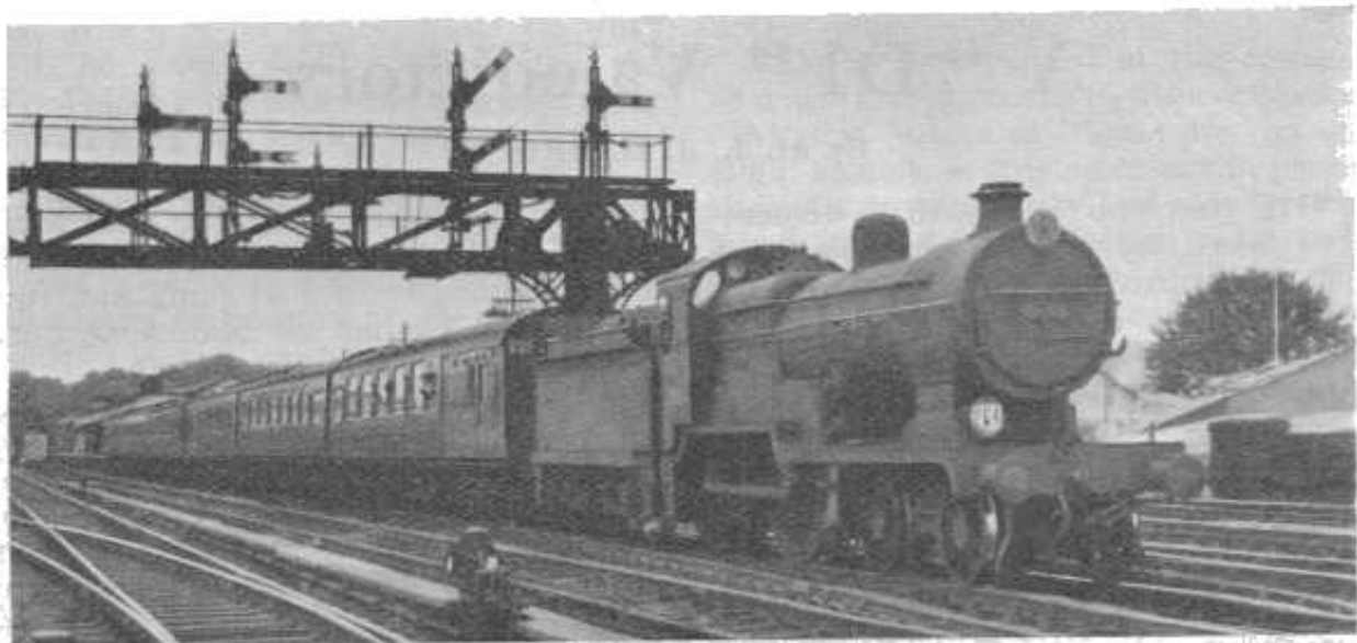
The 7.24 a.m. London Bridge to Ramsgate train leaving Ashford in May, 1959, headed by "D1" class 4-4-0 locomotive No. 31509
